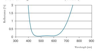
BBAR 宽光谱增透膜 可见波长段: R avg. < 0.5% at 400nm - 700nm (每镀膜面)
