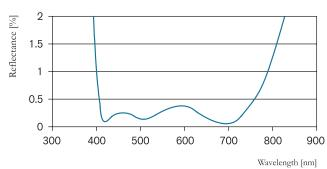
BBAR 宽光谱增透膜 可见波长段到近红外波长段: T avg. > 98% at 400nm – 900nm
